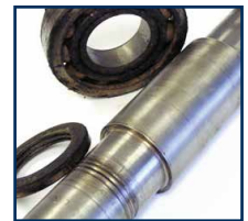
Shaft damage from a labyrinth seal
