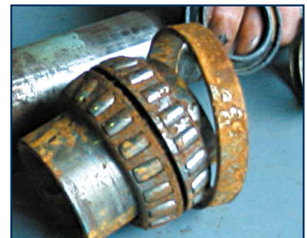
Moisture contaminated bearings
