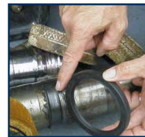
Shaft damage from a lip-seal
